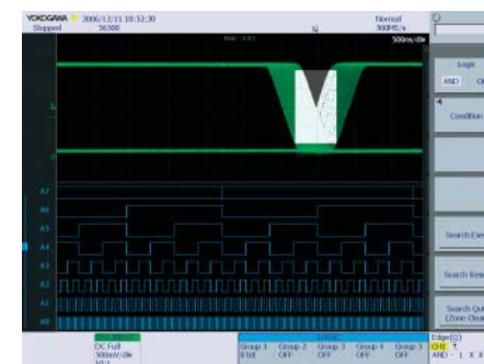
Zone search in History Memory Define 1 to 4 zones and search for waveforms that fall inside or outside the zone (s).
