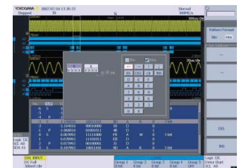
Serial bus Search for portions of analysis results of the logic signal's source serial bus that match specified conditions.
